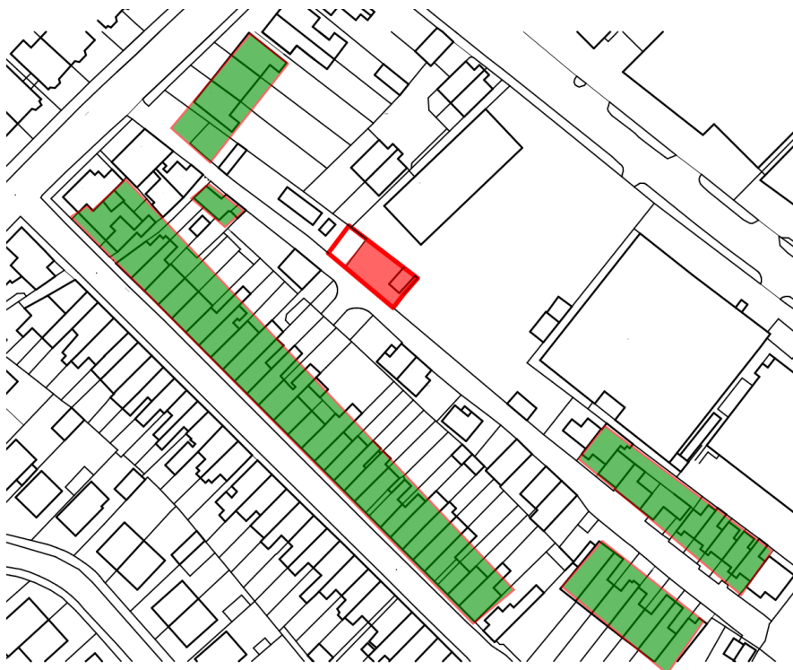
Extract of location plan showing dwellings locally that fill the width of their plots (not to scale)
