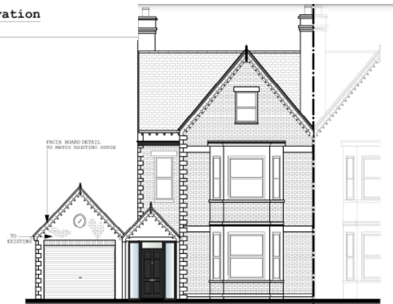
PR 03 Proposed Front Elevation 1:100 @ A3
