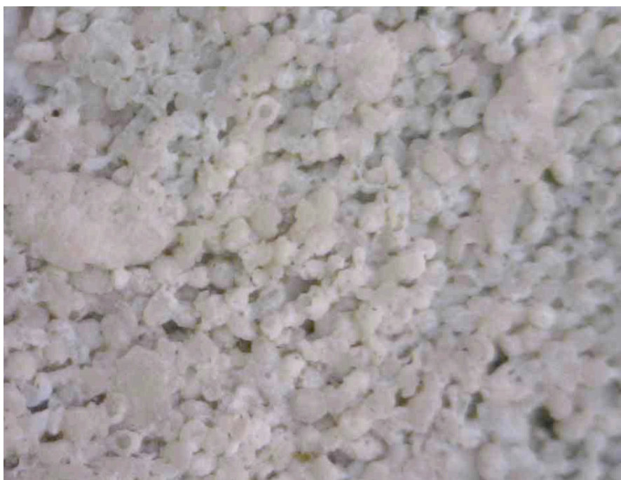
Fig 16: detail of stone (x50 magnification) showing how cleaning has opened up the surface pores of the stone
