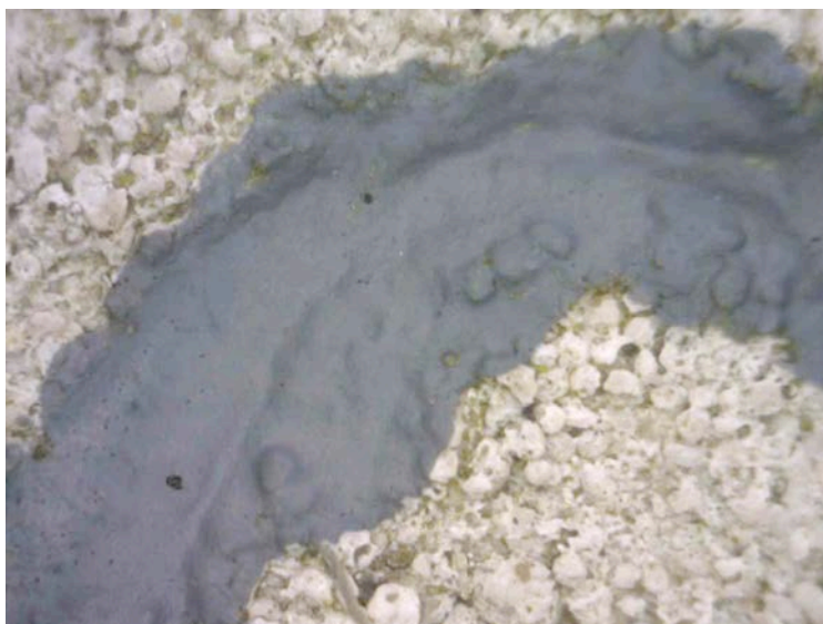
Fig 41: detail of repainted lettering (x50 magnification) showing inaccuracy of line compared to precision of original (see Fig 36)
