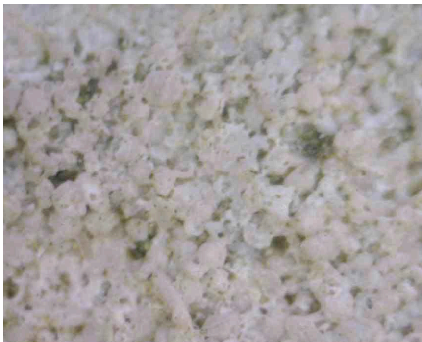
Fig 17: detail from north inscription panel showing how microbiological growth (green) has colonized deep within the pores of the stone
