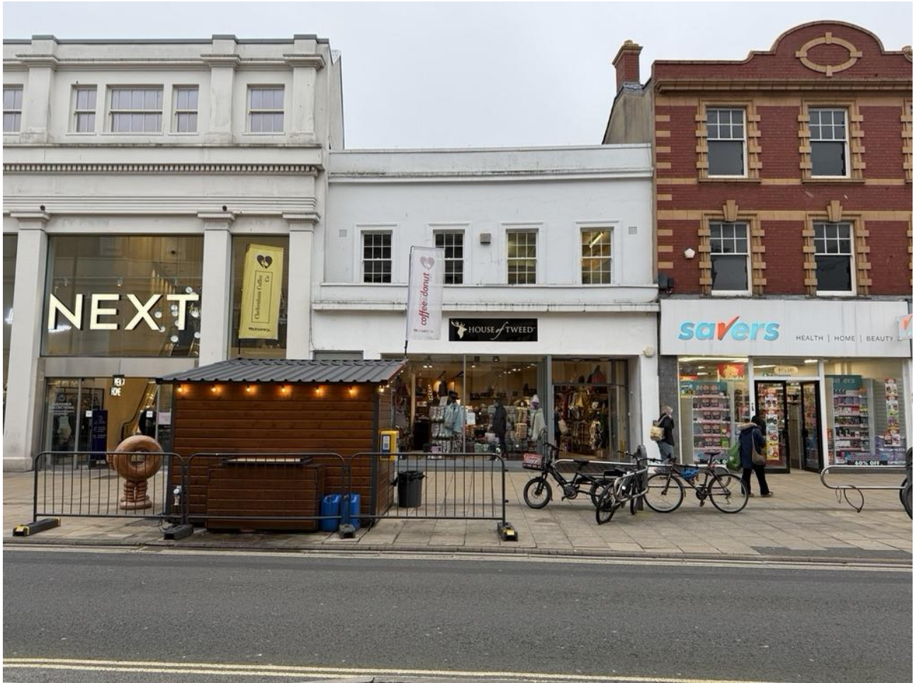
Barrier Fence extends past stall 7 f in either direction so the public can not walk out in to the road with a blocked line of sight. Barrier is attached to the stall.
