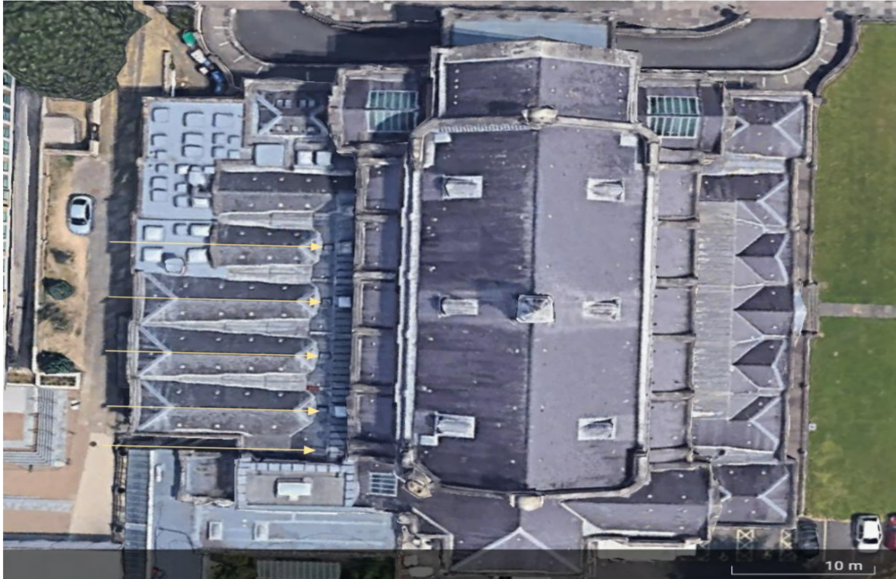
Figure 1. Aerial view of the Town Hall. Yellow arrows point to the location of the five skylights to be removed and slated over.
